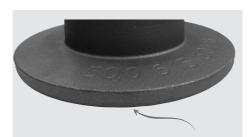
The result after about half a year of project work: The brake disc is cast burr-free due to modified feeder connection and gate geometry.
